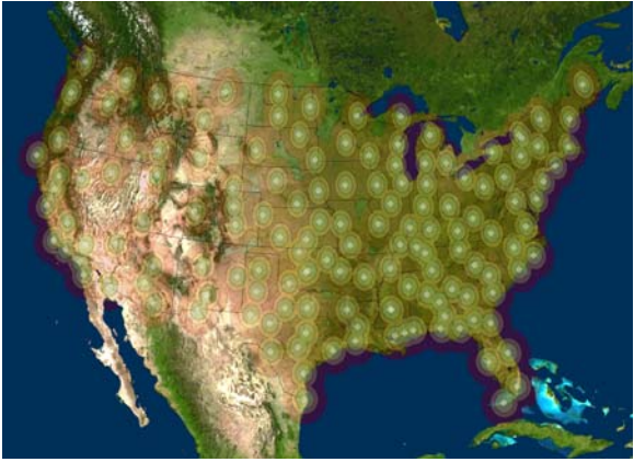
Figure 1 – The Nexrad network with range bubbles of 80km (green), 120km (yellow) and 200km (red).
